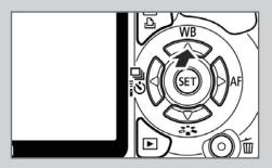
Please select the custom WB with the set-button and confirm the chosen picture with the set-button. We recommend naming the white balance picture taken with the DELTA® 20 T/DELTA® 20 Plus/DELTA® 20 accordingly.
